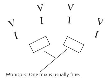
V = Vocal Mic Shure SM 58 or Equivalent I = Instrument Mic Shure SM 57 or Equivalent
